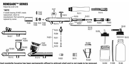
NOTE: Attached nozzle/tip housing has been permanently affixed to airbrush shell and is not made to be removed.
